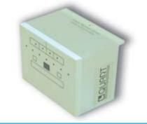
The QUART Biopsy Phantom is designed for regular QA/QC at stereotactic biopsy systems in digital and analogue mammography. Its design is optimised for all common image formats and fields-of-view (FoV) from 4x4cm. The phantom's integrated test objects are laid out for comprehensive QA/QC testing.
